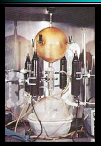
The Miller-Urey experiment attempted to recreate the chemical conditions of the primitive Earth with an atmosphere of methane, ammonia, and hydrogen, exposed to electrical discharges – an environment from which amino acids were formed – 1953, U of Chicago
